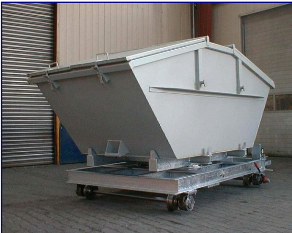
Trolley for longitudinal shifting of open top containers
