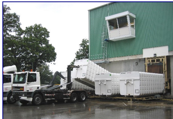
Traversing shifting device with four PM containers
