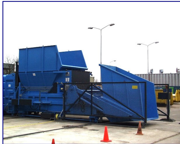
Traversing system for static compactor with special tipping device
